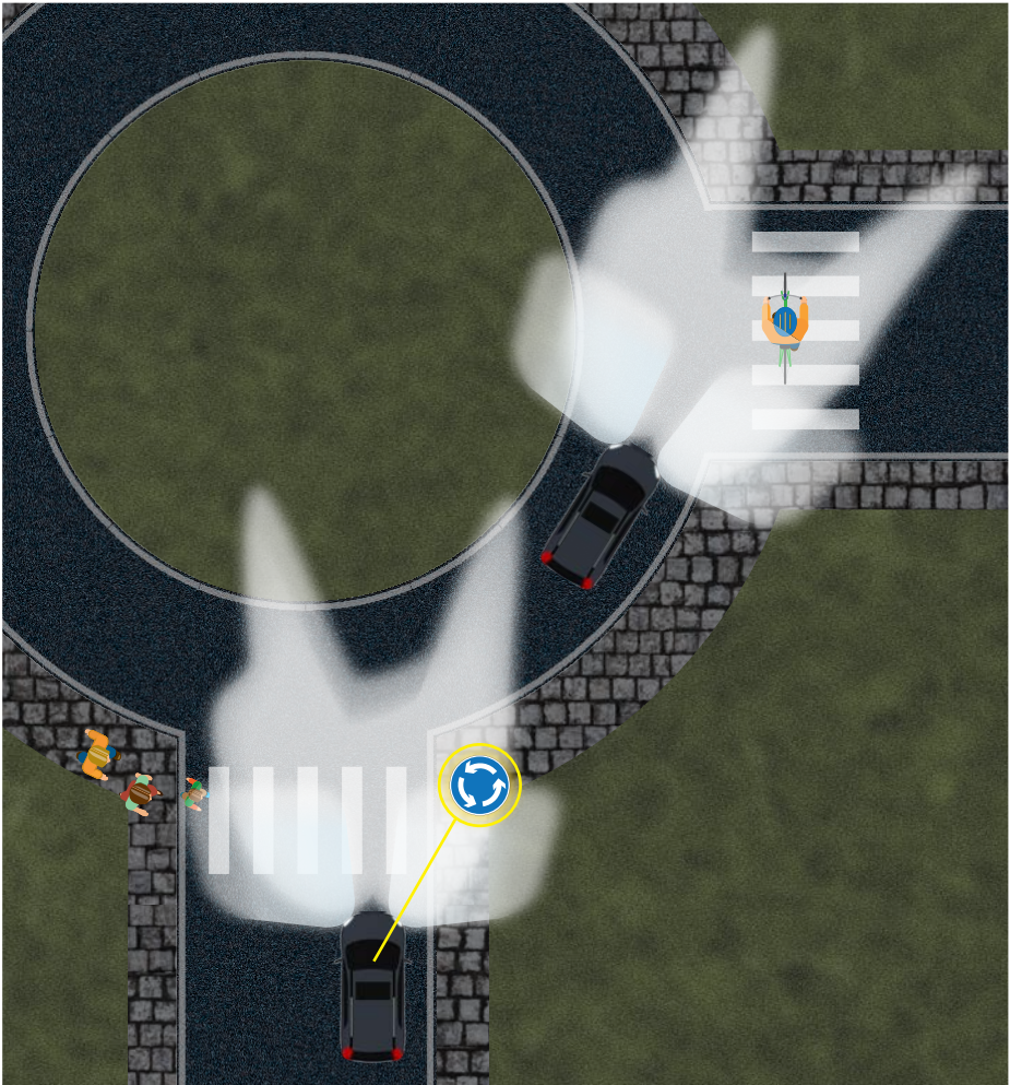
Ford is developing a Camera-Based Advanced Front Lighting System that can recognise certain traffic signs and widens the beam at junctions and roundabouts to better illuminate hazards that are not in the direction of travel.
