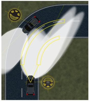
Ford's Camera-Based Advanced Front Lighting System uses GPS information and a forward-facing camera to better illuminate bends and dips on a chosen route, with the navigation system storing the road information.
