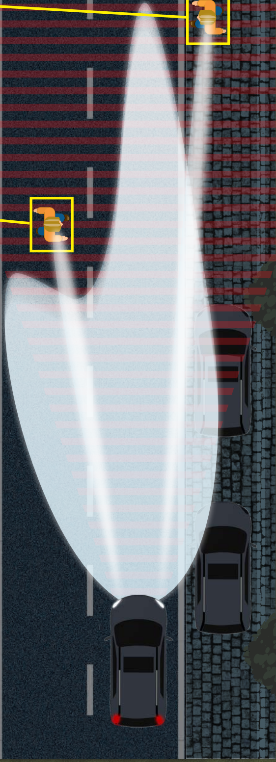
Ford is developing Spot Lighting technology that uses an infra-red camera to detect pedestrians, cyclists and animals. Spot Lighting highlights these hazards with specially designed headlights and also places them on the screen inside the car.
